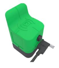
Eversensor (above) connects to harvesting source (below, thermoelectric generator) via a USB-C cable.
